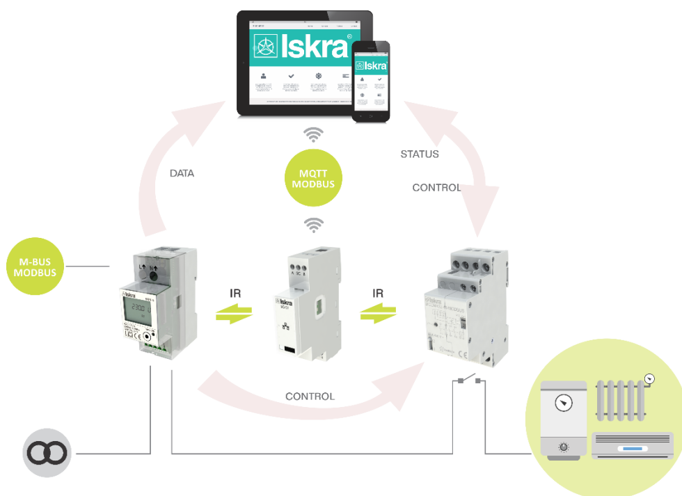
Figure 2: Connection diagram for SG. It is connected to an energy meter (on the left side of the SG) and to latching switch (on the right side of the SG) by IR communication. It is possible to read and control data with the computer or mobile phone.
